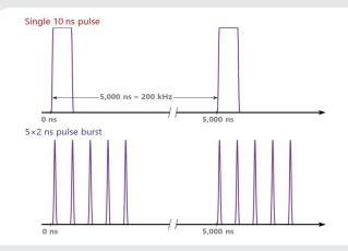
Figure 1. In burst mode, the laser emits a short series of pulses (burst subpulses) rather than an individual pulse. Each pulse burst can have nearly the same total energy as a single (longer) pulse at that same repetition rate.
