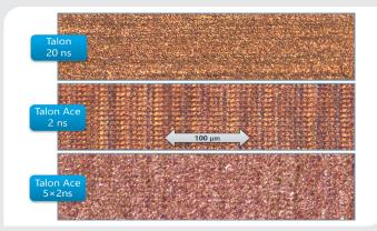
Figure 3. Closeup optical microscope photos showing machined surface quality for 2- and 20-ns single pulse outputs as well as a  $5 \times 2ns$  burst output.
