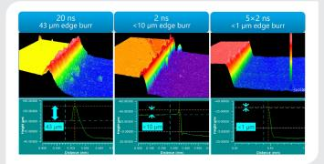
Figure 4. Optical surface profilometry reveals decreasing edge burr when going from 20 to 2 ns pulse widths, and further reduction with a  $5\times 2$  ns burst output.
