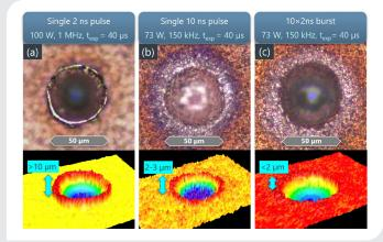
Figure 5. : For equal or lower average power, a  $10 \times 2$  ns burst offers superior results for flex PCB top copper via opening compared to single 10 ns and 2 ns pulses.
