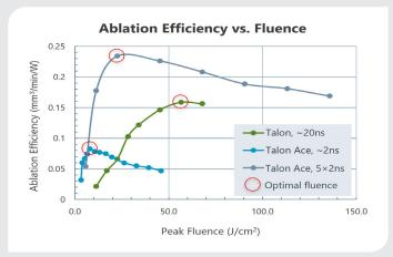
Figure 2. Ablation efficiency data illustrates the importance of pulse width and the benefit of using pulse bursts when processing copper.
